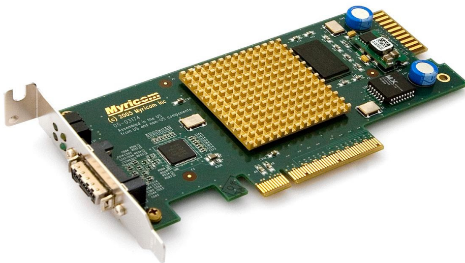
Dual-protocol Myri-10G NIC with a PCI-Express x8 host port and a 10GBASE-CX4 network port.
